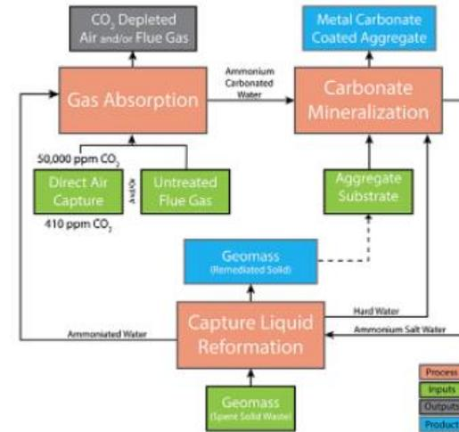
The capture solution reacts with the Geomass, reforming it, these metal ions are released and combined with the carbonate solution to form the carbonate mineral coating.
