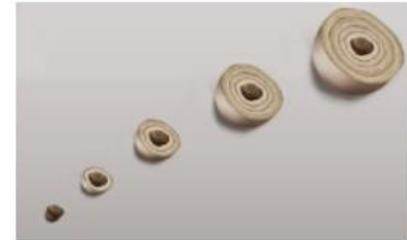
A rock particle is coated with our synthetic limestone, forming a carbon-sequestering coating that is 44% by mass CO<sub>2</sub>. The coating can contain residual fine particles from the capture solution regeneration.
