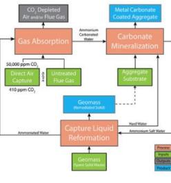
capture solution reacts with the Geomass, reforming it, these metal ions are released and combined with the carbonate solution to form the carbonate mineral coating.
