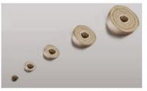
A rock particle is coated with our synthetic limestone, forming a carbonsequestering coating that is 44% by mass CO2.The coating can contain residual fine particles from the capture solution regeneration.
